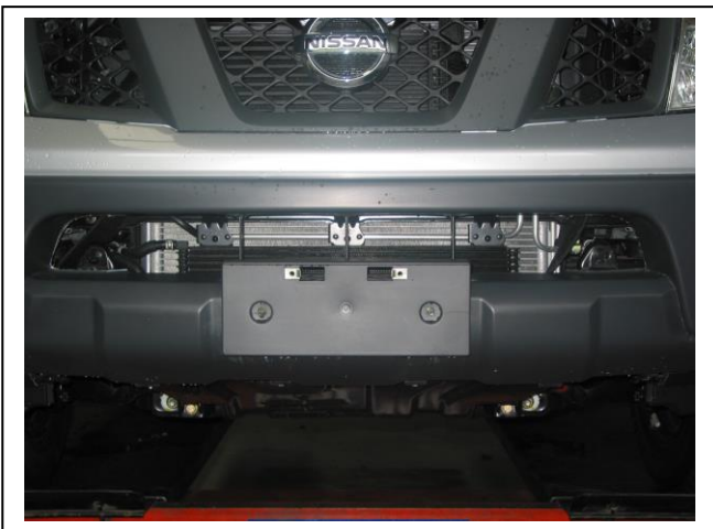
Figure 5 – Navara D40 Only – After section is trimmed
